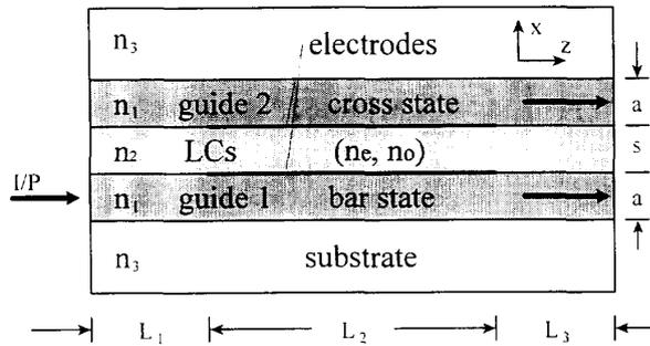
Fig. 1. The device configuration we proposed is shown here. It consists of two normal waveguides fabricated on two substrates respectively, a pair of electrode on the two waveguides, and a thin LC's layer separating the two guides.
