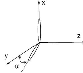
Fig. 2. Two states of NLC's are illustrated. One is molecular parallel to the guiding layer surface but with a pretilted angle  $\alpha$  to the  $y$  axis; another is molecular normal to the surface and parallel to the  $x$  axis.
