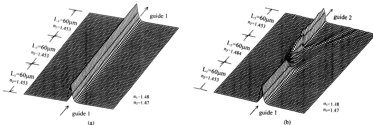
Fig. 4. (a) The bar state: power is confined in waveguide 1 and no coupling occurs; (b) The crossover state: power in waveguide 1 is coupled to another one, where  $L_1 = L_2 = L_3 = 60 \mu\text{m}$ .
