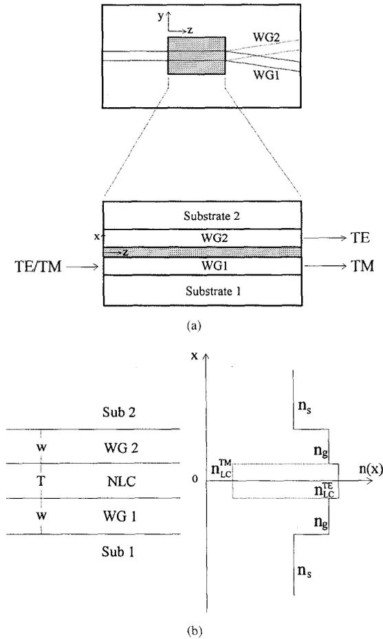
Fig. 1. (a) The schematic diagram of the proposed directional-coupler polarization splitter, which is composed of a pair of glass waveguides with an intermediate layer of nematic liquid crystal: the upper plot shows the top view of the whole device, while the lower one is the cross-section view in the coupling region. (b) The corresponding refractive index profile in the coupling region.
