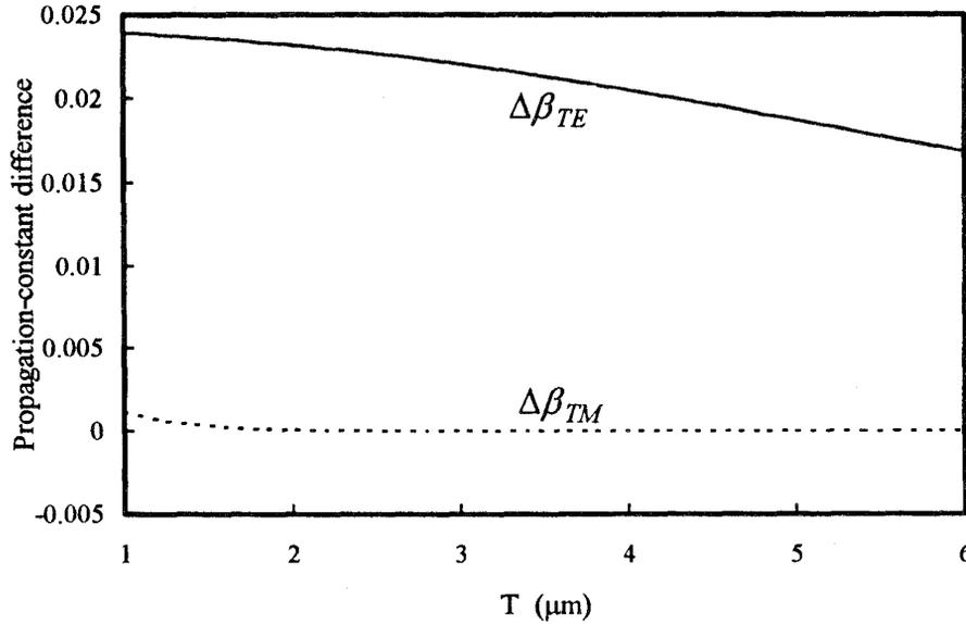
Fig. 3. The dependence of propagation-constant differences between the two normal modes on  $T$ : the solid and dotted lines correspond to the  $\Delta\beta_{TE}$  and  $\Delta\beta_{TM}$ , respectively. The waveguide parameters are  $n_{LC}^{TE} = 1.530$ ,  $n_{LC}^{TM} = 1.380$ ,  $n_g = 1.526$ ,  $n_s = 1.512$ , and  $w = 3.52 \mu\text{m}$ .
