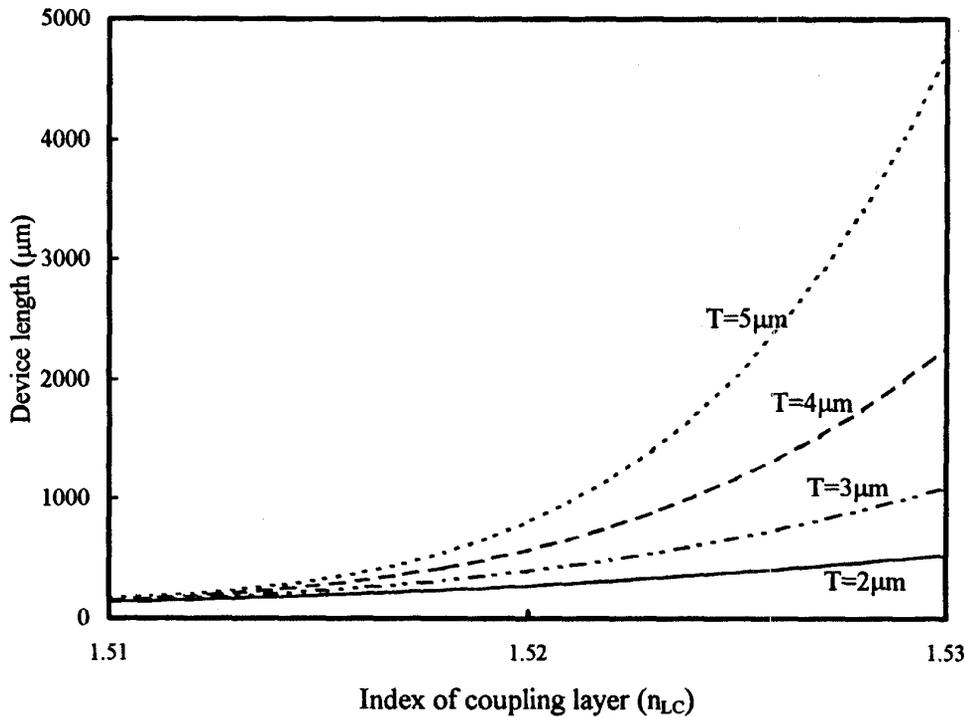
Fig. 4. The calculated device length as a function of  $n_{LC}^{TE}$  for various NLC layer thickness  $T$ . Assume that  $n_g = 1.526$  and  $w = 3.52 \mu m$ .
