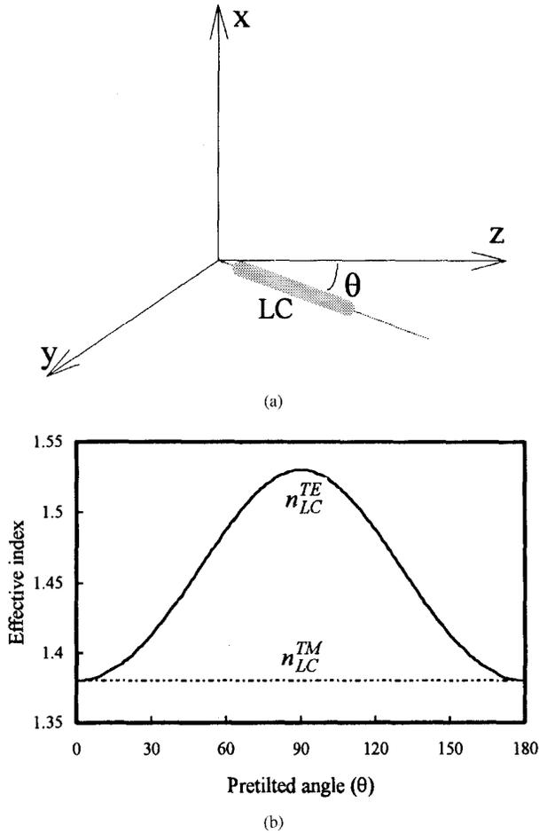
Fig. 2. (a) The orientation state of NLC, assuming that the molecular axis is aligned along the direction parallel to the waveguide surface and with a pretilted angle  $\theta$  to the light propagation. (b) The effective indexes seen by the TM and TE modes as a function of the pretilted angle  $\theta$ : the solid and dotted lines correspond to the  $n_{LC}^{TE}$  and  $n_{LC}^{TM}$ , respectively.
