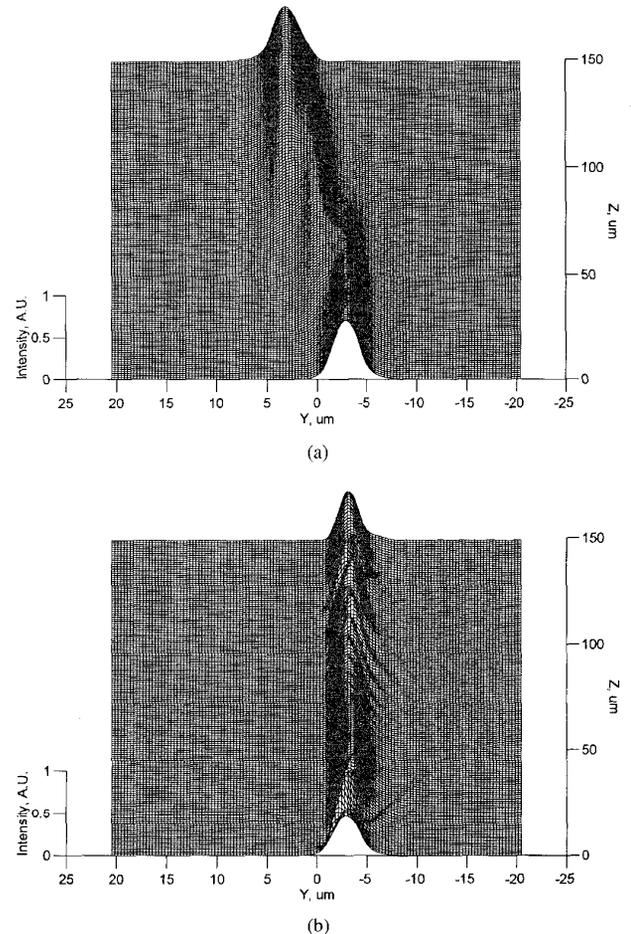
Fig. 7. The BPM simulated field evolution along the directional coupler of (a) TE mode and (b) TM mode.
