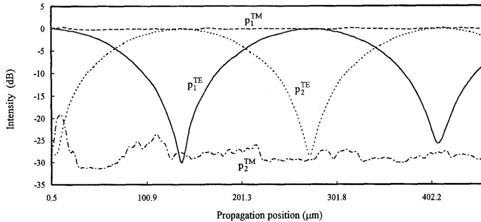
Fig. 6. Propagating behaviors of this polarization-splitting coupler. The solid, dotted, dot-dashed, dashed lines, respectively, correspond to power evolution of the  $P_1^{\text{TE}}$ ,  $P_2^{\text{TE}}$ ,  $P_1^{\text{TM}}$ , and  $P_2^{\text{TM}}$  along the directional coupler.
