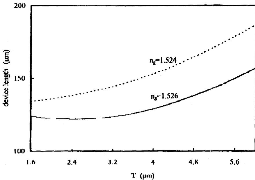
Fig. 5. The influence of  $T$  on the device length  $L_d$ , calculated for  $n_g = 1.524$  (dotted line) and  $1.526$  (solid line) with  $w = 3.52 \mu m$  and  $n_{LC}^{TE} = 1.530$ .
