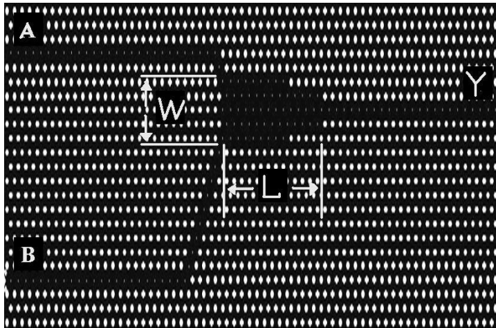
Figure 2、 Schematic diagram of the proposed XOR optical logic gate.
